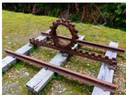
West Coast Wilderness Railway rack and pinion model
